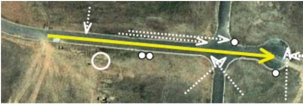
Fig. 1 Human paths (dashed line), mannequin locations (solid circles), Suburban path (solid line), and random human motion (open circle) on the test course.
