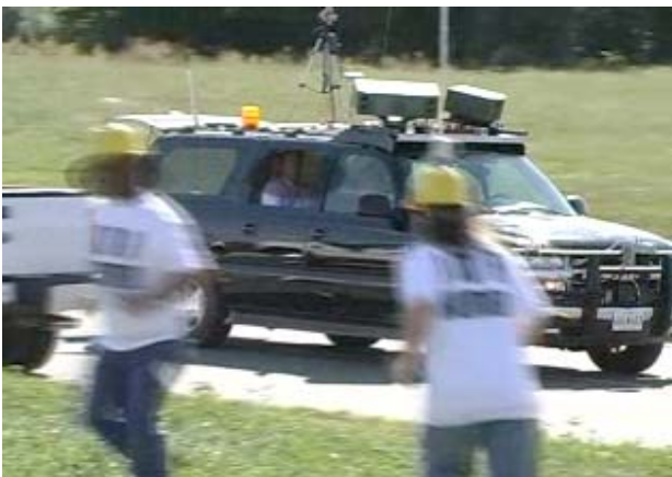
Fig. 2 Suburban equipped with sensors and algorithm processors (shuttles) passes a truck and jogging humans.
