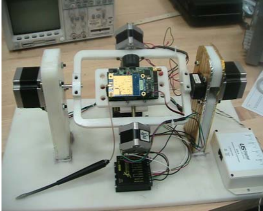
Fig. 5. Autopilot on hardware-in-the-loop simulation gimbal
