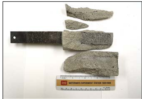
Fig. 2. Photo of coated strap in mortar cylinder after breaking the cylinder by withdrawing the strap. Note the mortar still adheres to the coating.
